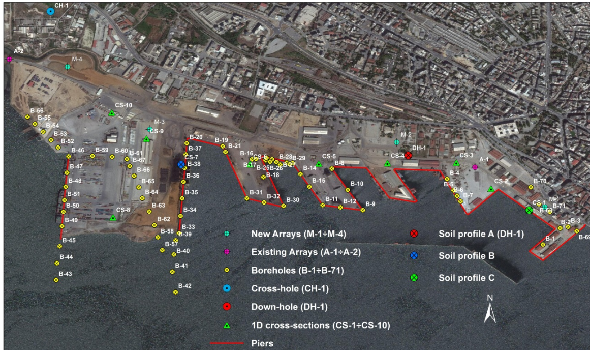
Fig. 6.3 Location of the sampling boreholes, down-hole and cross-hole tests, microtremor measurements and 1D cross-sections of the broader Thessaloniki port area. The location of the new field microtremor measurements (M-1, M-2, M-3, M-4) are also shown.
