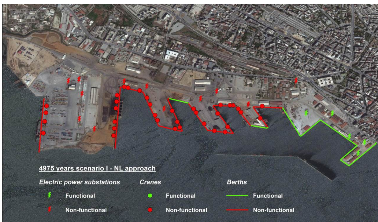
Fig. 6.34 Spatial distribution of the components functionality for the 4975 years scenario I- NL approach
