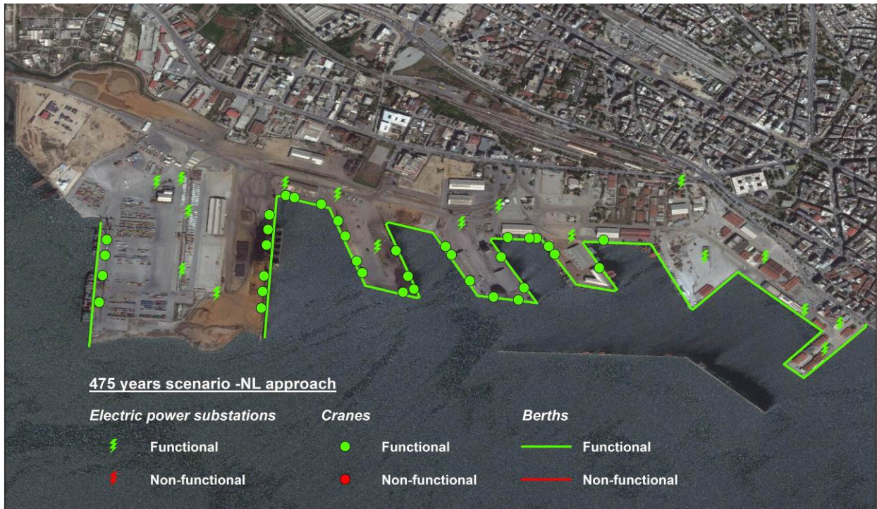
Fig. 6.32 Spatial distribution of the components functionality for the 475 years scenario - NL approach
