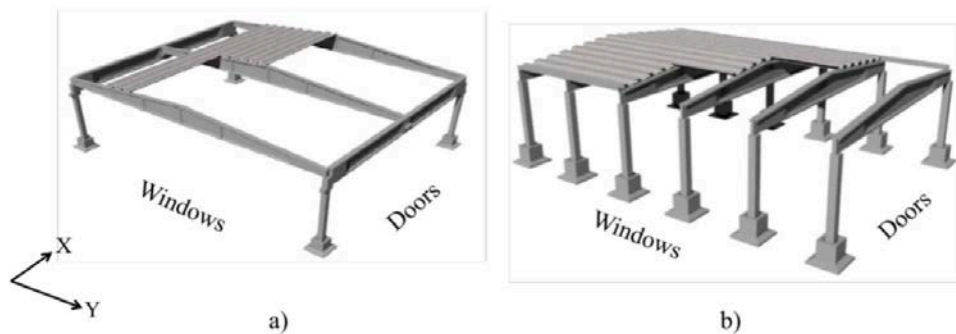
Fig. 7.2 Structural configuration and assumed position of openings in a) Type 1 and b) Type 2 industrial building (Casotto et al., 2015)
