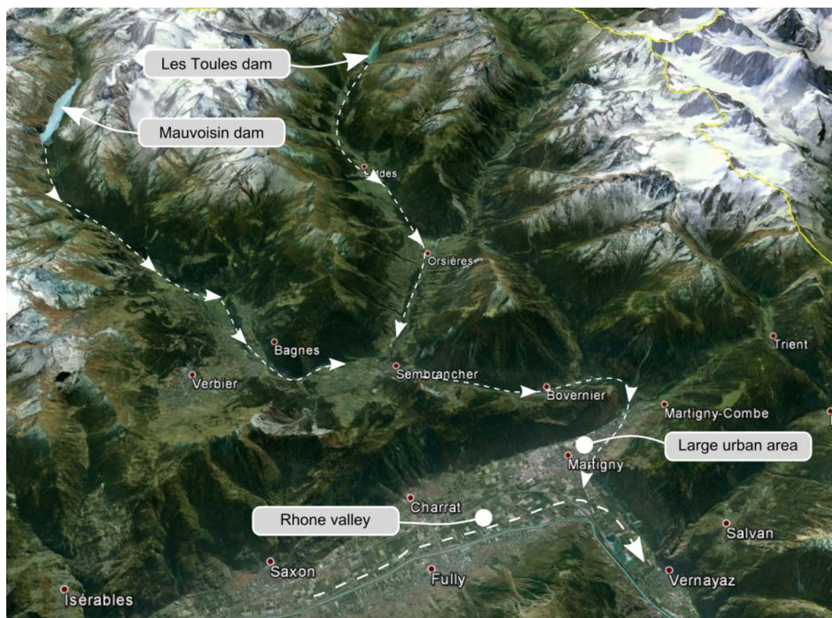
Fig. 3.2 Implementation of two large Alpine dams in Switzerland: Les Toules and Mauvoisin. Both are placed in tributaries of the Rhone River and, in the event of a failure, the main urban areas where losses could be expected are relatively far downstream. Neither of these dams is analyzed in this document
