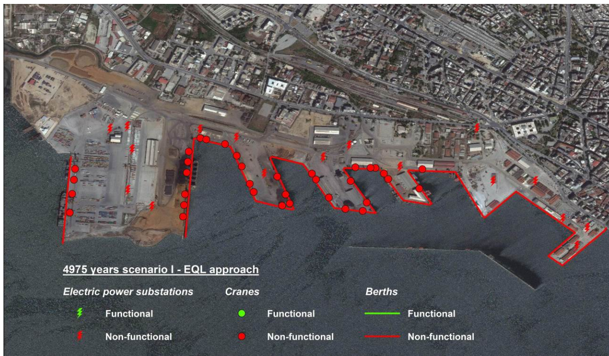
Fig. 6.33 Spatial distribution of the components functionality for the 4975 years scenario I- EQL approach
