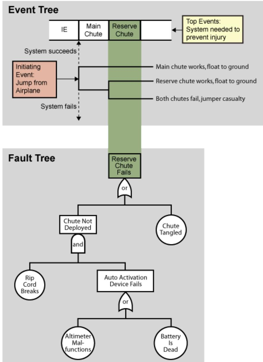
**Fig. 1.1 Event and fault tree example (USNRC 2012)**
