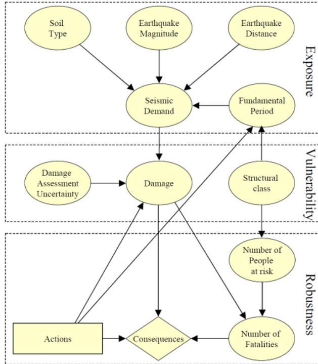
Fig. 2.3 BN framework for seismic risk management (source: Bayraktarli et al., 2005)
