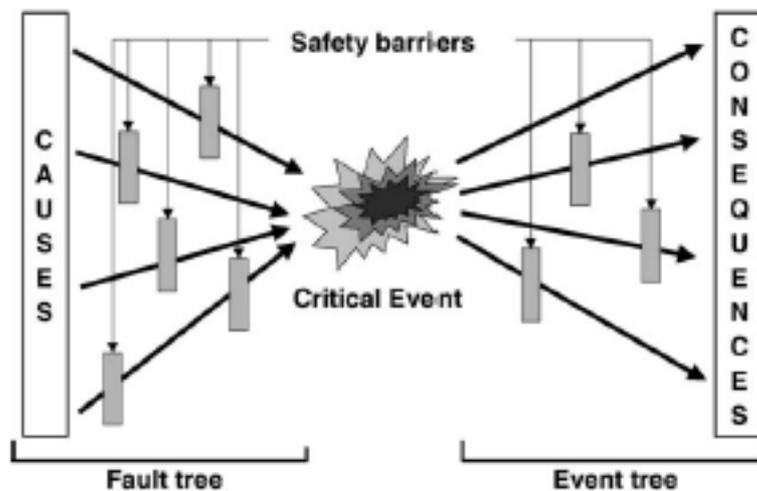
**Fig. 1.2 Bow-tie critical event model with safety barriers [ARAMIS project (De Dianous and Fiévez 2006)]**
