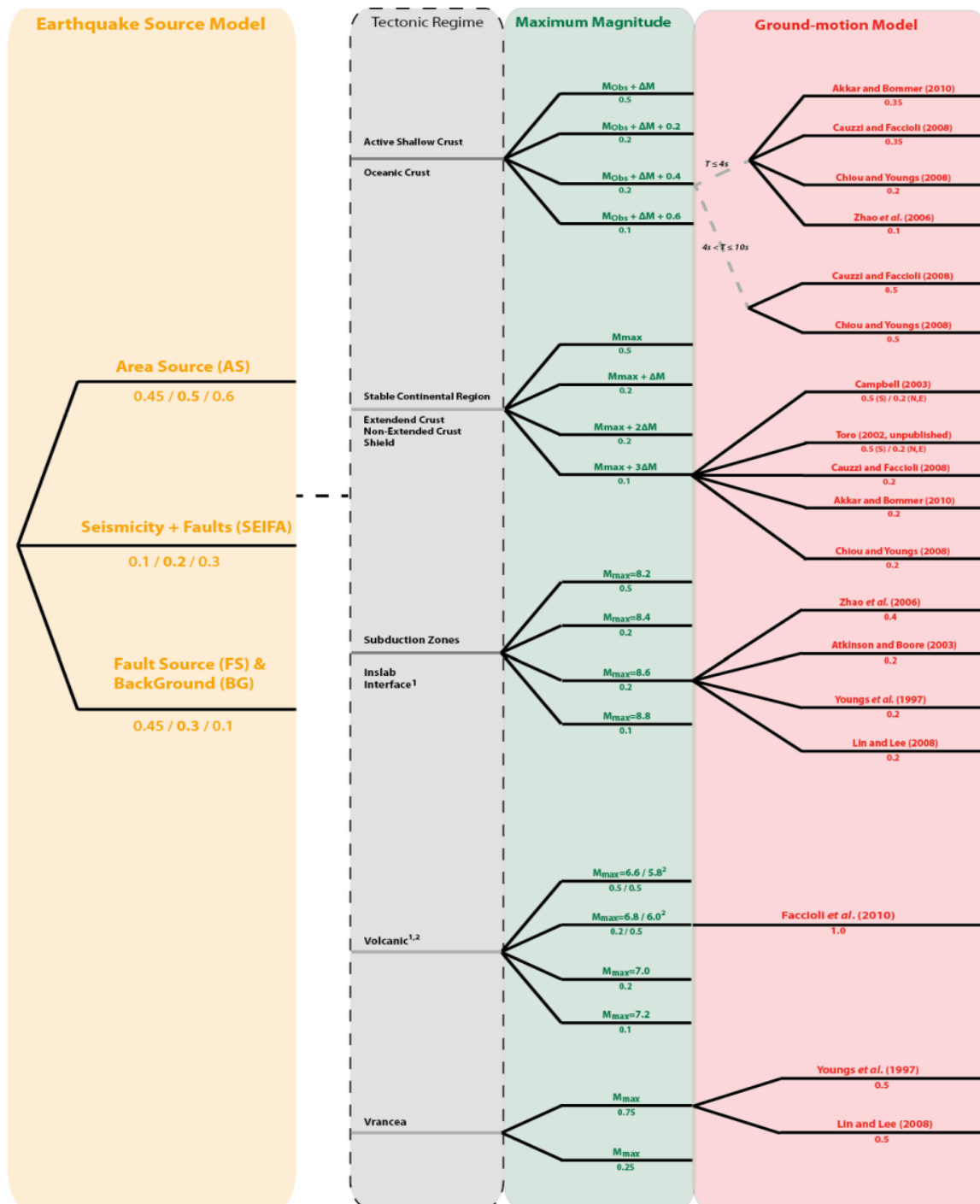
Figure 2-4: SHARE logic tree. Colours depict the branching levels for the earthquake source models (yellow), maximum magnitude models (green) and ground motion models (red). Values below the black lines indicate the weights, for the source model these indicate the weighting scheme for the different return periods. Tectonic regionalization is not branching levels (grey) of the model; however, it defines the GMPs to be used (from Woessner et al., 2013, Giardini et al. 2013).
